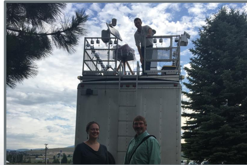
Collocation of Purple Air sensors with reference monitors at the USFS Fire Science Lab
