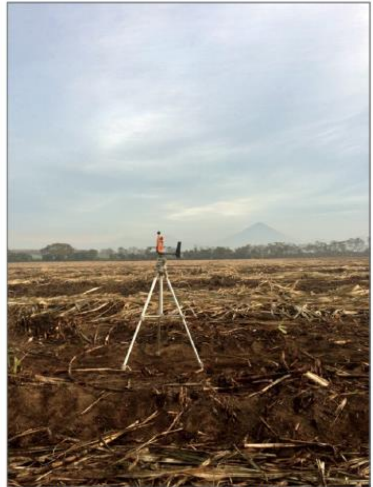
Wet-Bulb Globe Temperature Monitor in a Sugarcane Field in Guatemala during a Research Data Collection Day.
